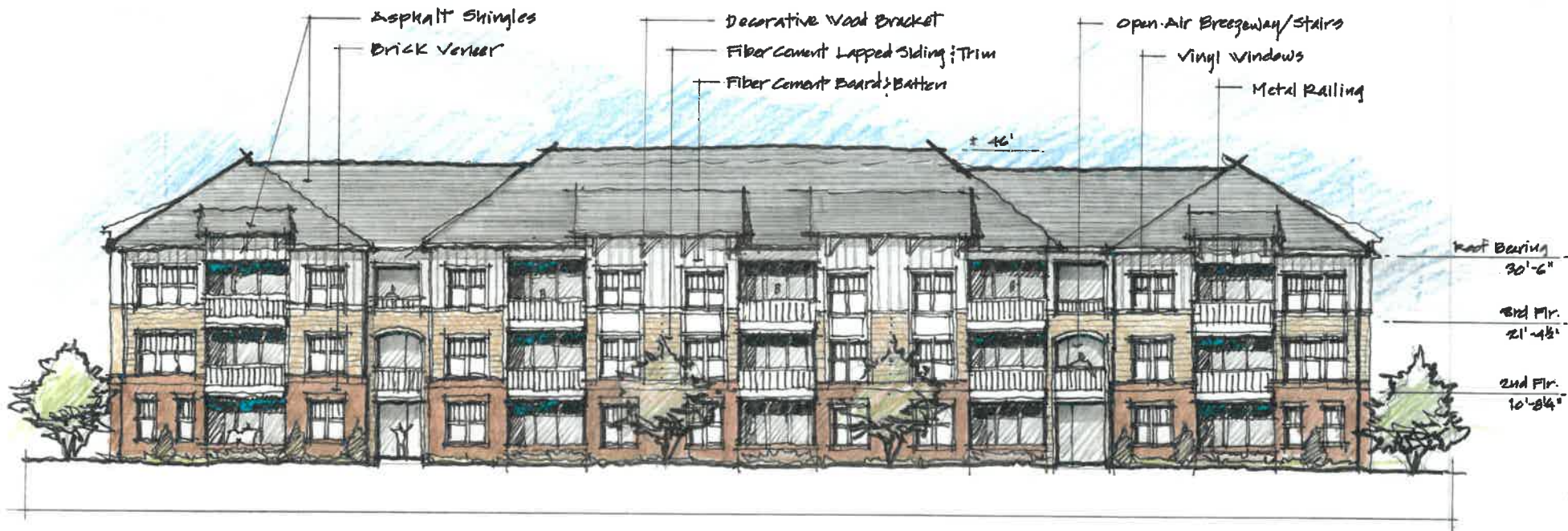
BUILDING 'C'. Front Elevation
